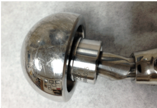
Fig. 1 Modularity can be the weak point in the implant design and the source of more debris from corrosion.
